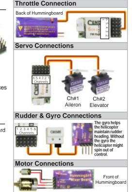
The mixer speed controller controls the amount of power transfered to the main and tail motors in proportion.
